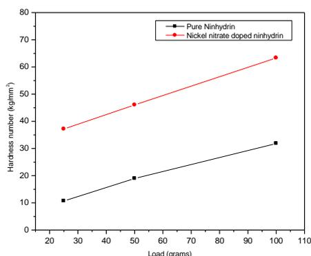
Fig.6. Plot of hardness vs load for pure and nickel doped ninhydrin crystals.
