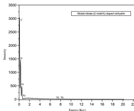
Fig.5. EDAX spectrum of Nickel nitrate doped ninhydrin samples
